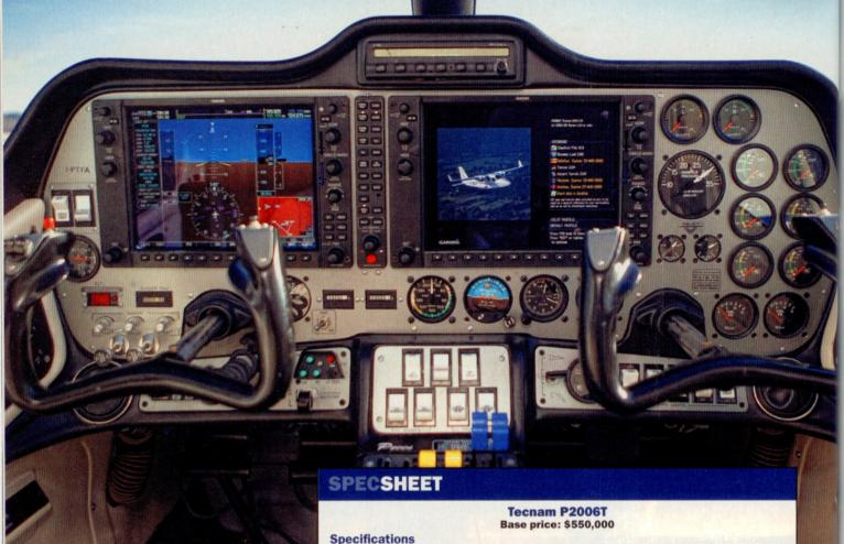
of manifold pressure and saw 151 KTAS. A 75-percent power setting of 25 inches of manifold pressure yielded a 142 KTAS cruise speed—a few knots faster than book. This, at 3,500 feet and a cool minus 8 degrees Celsius.
